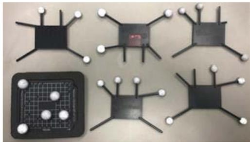
**Figure 1.** Reflective markers for rigid body tracking.
