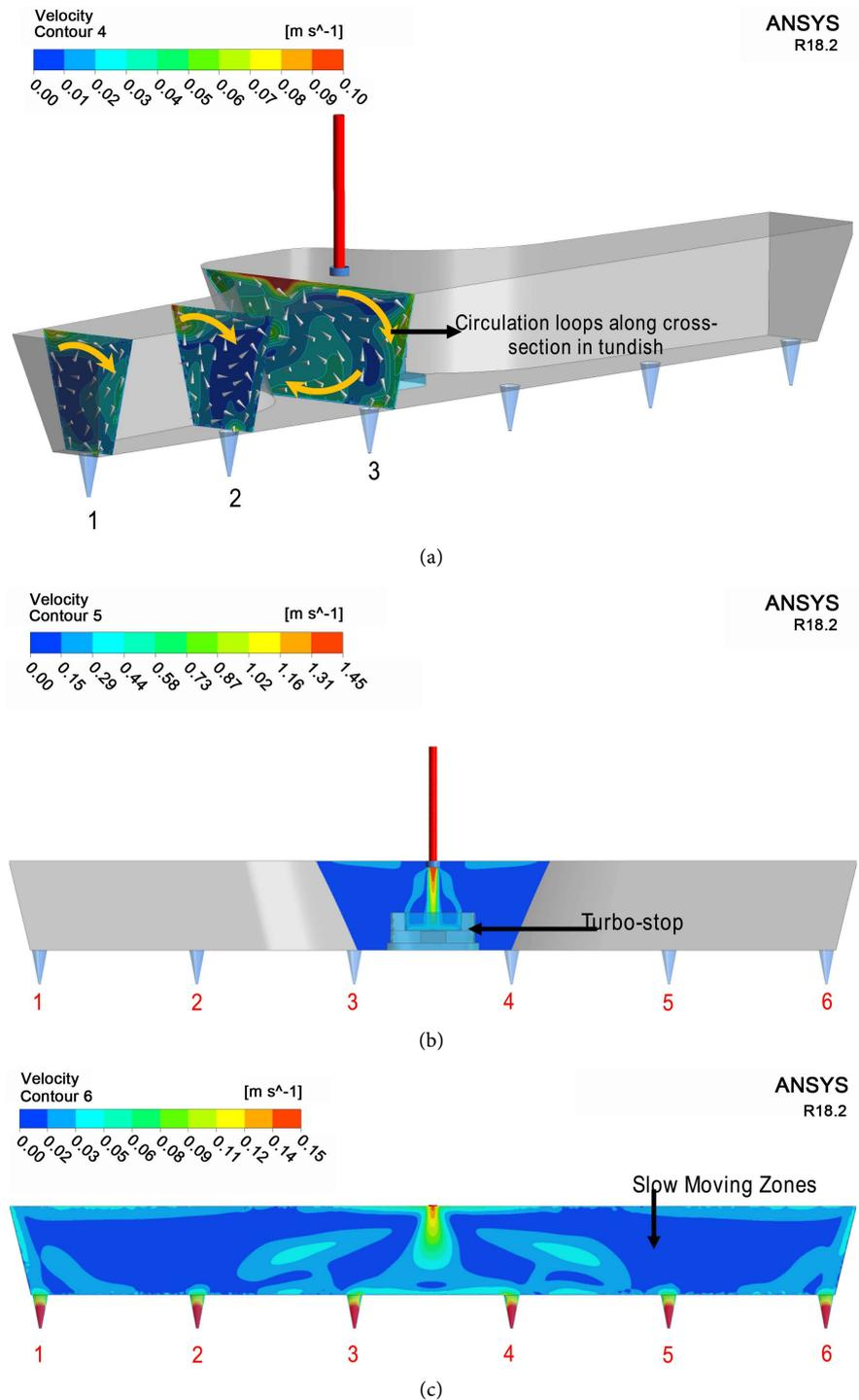
**Figure 4.** Velocity contours on various planes in 6 strands Tundish for all strands running. (a) Velocity field on a plane across the Tundish near three outlets for 6 strand Tundish; (b) Velocity field on a plane passing through the inlet for 6 strand Tundish; (c) Velocity field on a plane passing through all outlets for 6 strand Tundish.
