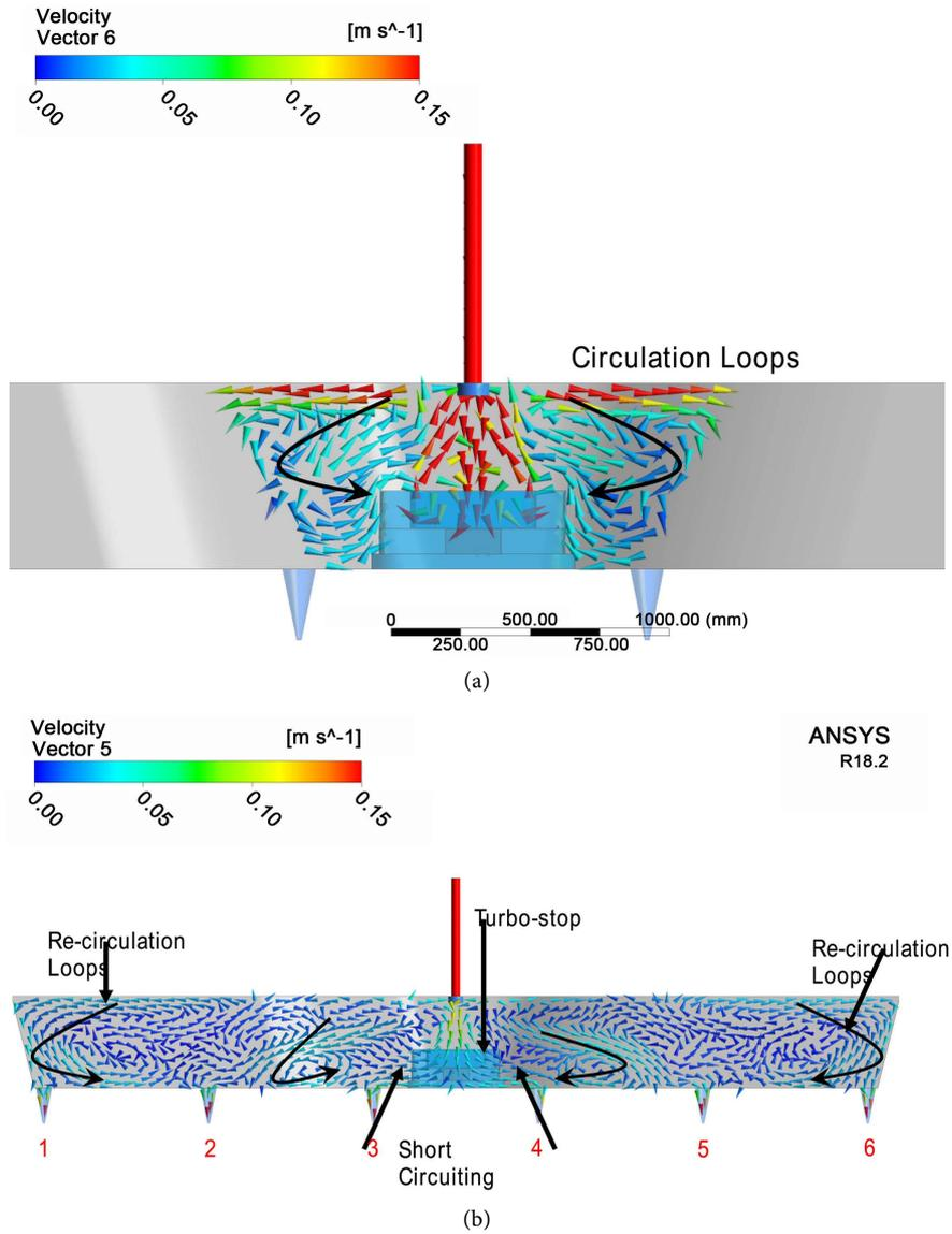
**Figure 5.** Velocity vectors at various locations in 6 strands Tundish all strand functional. (a) Velocity vector field on a plane passing through the inlet for 6 strand Tundish; (b) Velocity vector field on a plane passing through all outlets for 6 strand Tundish.
