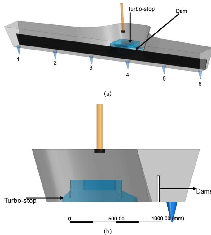
**Figure 15.** Tundish design with long baffle (Design 2). (a) Iso-view of Tundish with long dam; (b) Side view of Tundish with 1 long dam.
