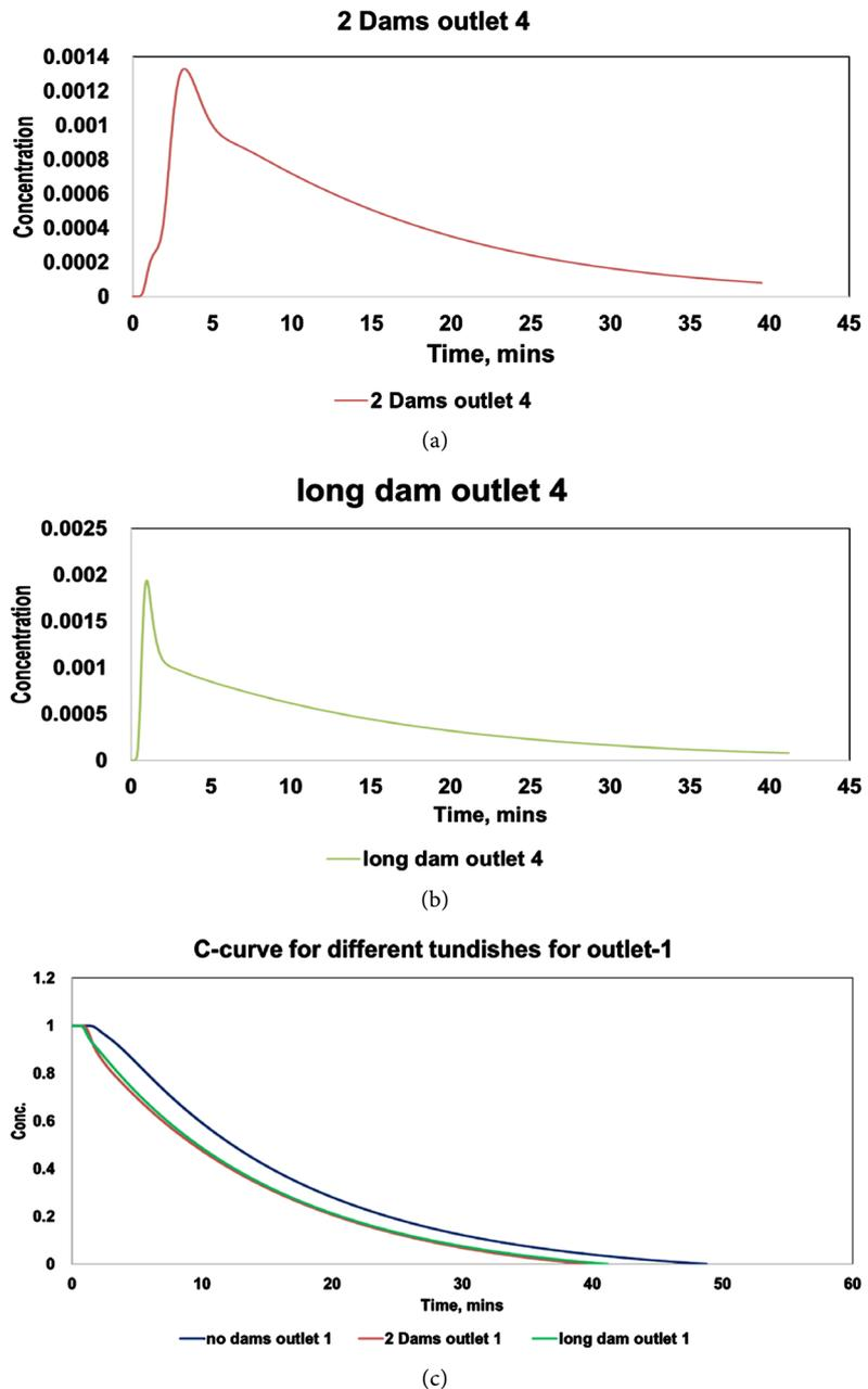
**Figure 16.** Effects of baffles on the performance of Tundish. (a) RTD curve for strands 1 and 4 for two baffle Tundish; (b) RTD curve for strands 1 and 4 for long baffle Tundish; (c) Transition time prediction for different Tundish designs (no dams, single long dam and 2 dams).
