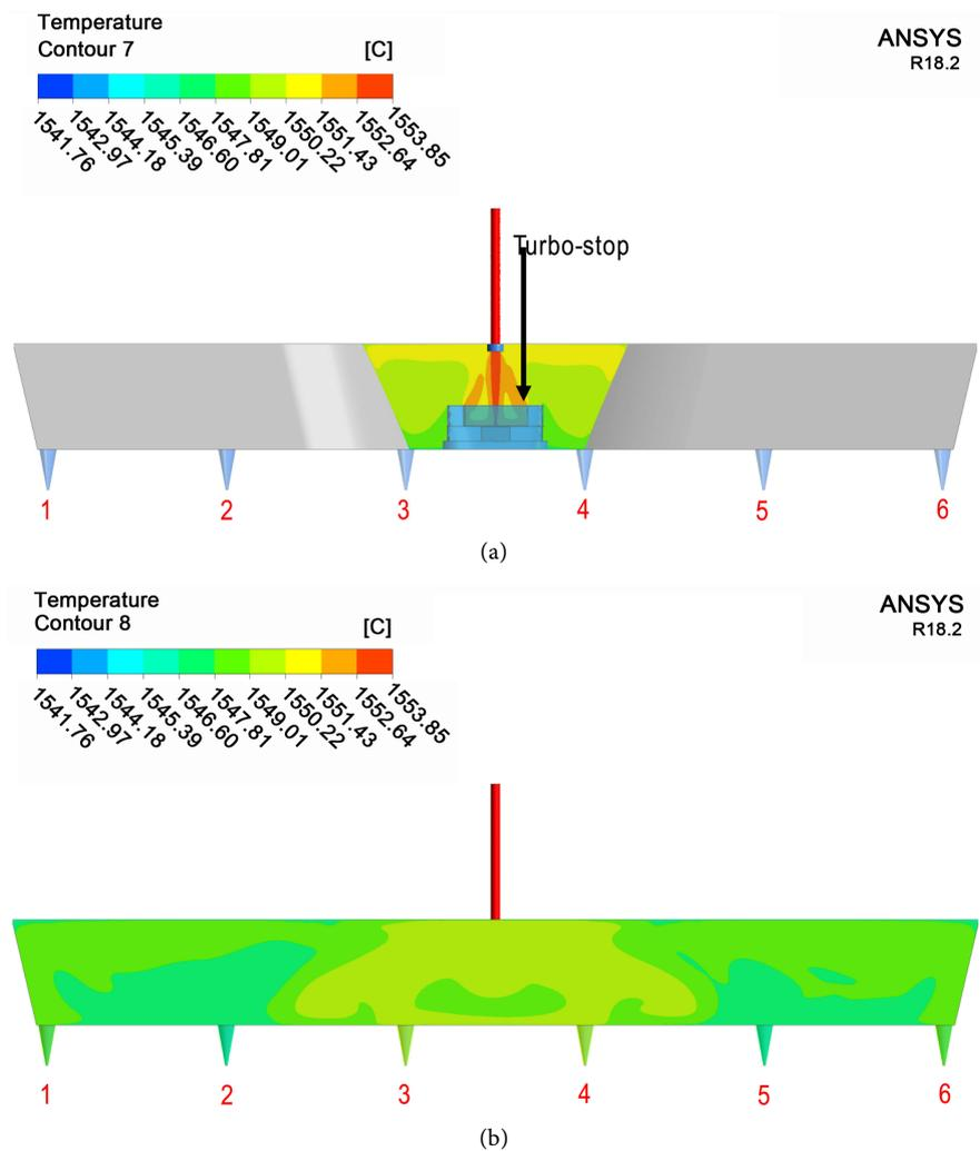
**Figure 7.** Temperature counters on various planes in 6 strands Tundish all strand functional. (a) Temperature field on a plane passing through the inlet for 6 strand Tundish; (b) Temperature field on a plane passing through all outlets for 6 strand Tundish.
