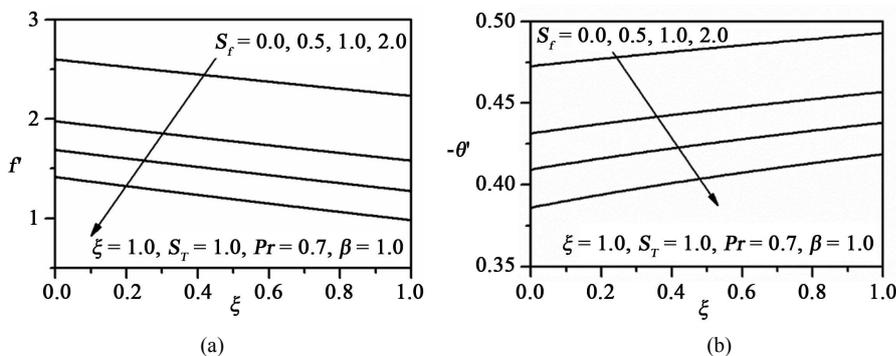
Figure 5. (a) Effect of  $S_r$  on the Skin-friction coefficient results; (b) Effect of  $S_r$  on the Nusselt number results.
