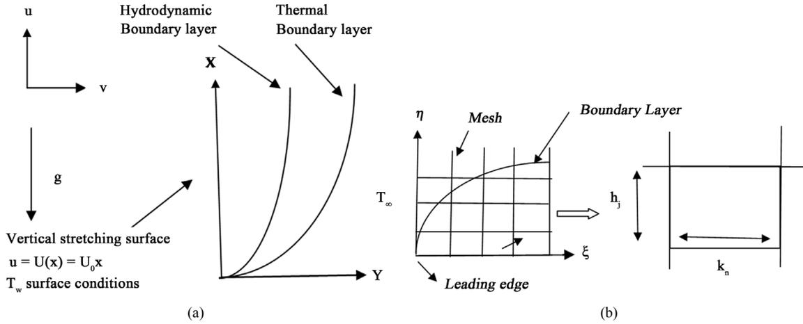
**Figure 1.** (a) Physical model and coordinate system; (b) Grid meshing and a Keller box computational cell.
