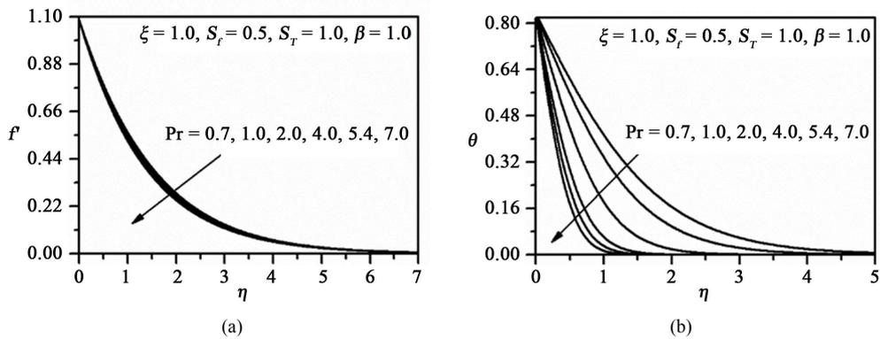
Figure 7. (a) Influence of  $Pr$  on the velocity; (b) Influence of  $Pr$  on the temperature.
