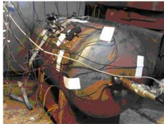
Specimen with gauges and sensors
