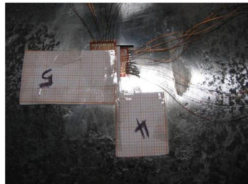
Instrumentation gauges (small defect)
