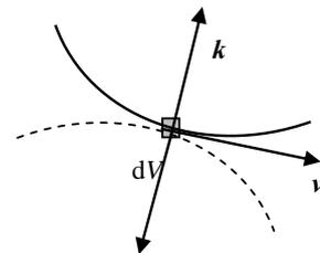
**Figure 1. Illustration of distinguishing the flow situations in infinitesimal surrounding of a flow field point ( $dV$ ) by the curvature  $k$  of the velocity fluctuation streamline passing this point: the flow situations with the same  $\mathbf{v}'$  but opposite  $k$  prove different.**
