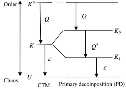
**Figure 3. Primary decomposition (PD) of the turbulence energy: the energy graphs of turbulent flow field for the situation assumed within the CTM and for the situation corresponding to (5).**
