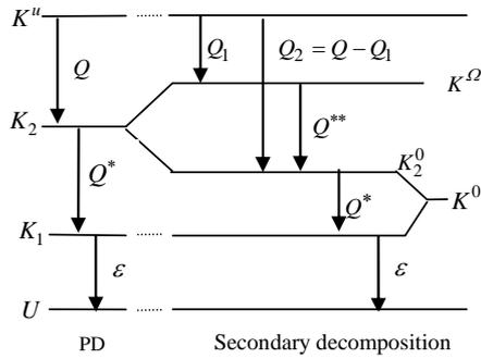
**Figure 4. Secondary decomposition of turbulence energy: the energy graphs corresponding to the PD and to the secondary decomposition.**
