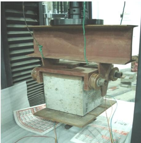
Figure 1. Concrete specimens and wedge splitting test.
