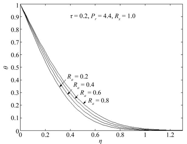
Figure 7. Temperature distributions  $\theta$  with  $P_r = 4.4$ ,  $\tau = 0.2$ ,  $R_x = 1.0$ .
