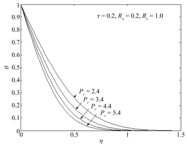
Figure 8. Temperature distributions  $\theta$  with  $R_a = 0.2$ ,  $\tau = 0.2$ ,  $R_x = 1.0$ .
