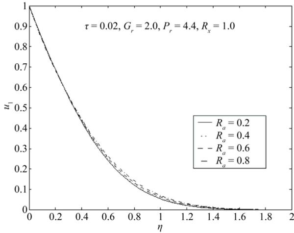
Figure 3. Velocity distributions  $u_1$  with  $G_r = 2.0$ ,  $P_r = 4.4$ ,  $\tau = 0.02$ ,  $R_x = 1.0$ .
