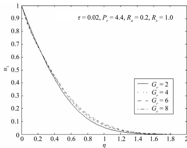
Figure 5. Velocity distributions  $u_1$  with  $R_a = 0.2$ ,  $P_r = 4.4$ ,  $\tau = 0.02$ ,  $R_x = 1.0$ .
