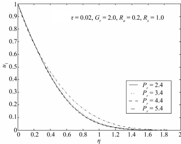
Figure 4. Velocity distributions  $u_1$  with  $G_r = 2.0$ ,  $R_a = 0.2$ ,  $\tau = 0.02$ ,  $R_x = 1.0$ .
