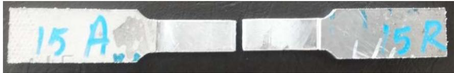
**Figure 8.** Photograph of tensile specimen fractured at the weld zone.
