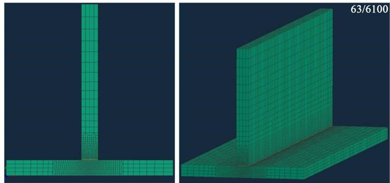
**Figure 2.** The 2D mesh created describing the cross-section of the T-joint to be modelled, and the resulting 3D mesh when swept through in to the welding direction. Image taken using ESI Visual Environment pre-processing software.
