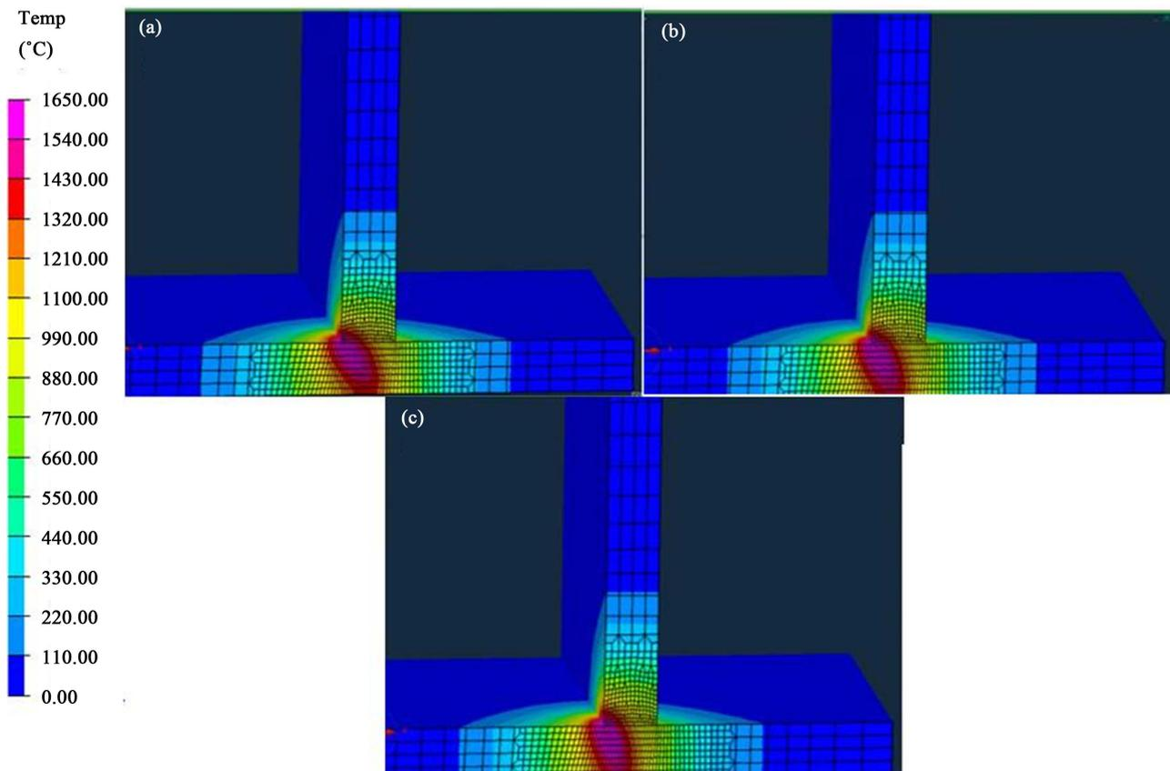
**Figure 3.** Variation in weld pool shape and angle, showing (a) the  $-8^\circ$  torch angle model; (b) the default model and (c) the  $+8^\circ$  torch angle model. (Images taken using Sysweld2014 computations and Visual Environment 9.5 post-processing software).
