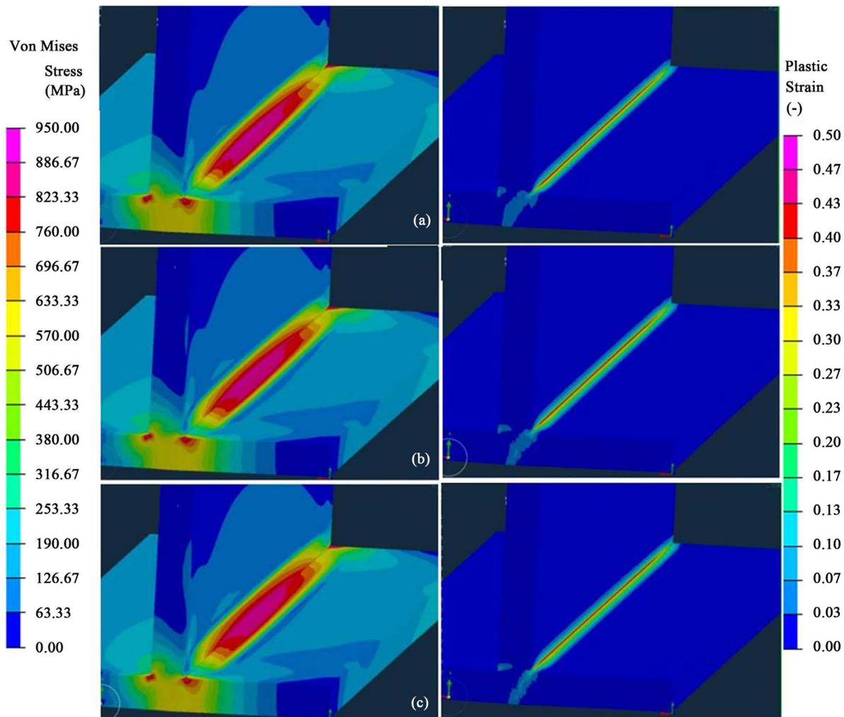
**Figure 7.** (left) Von Mises residual stress distribution, and (right) plastic strain distribution from the T-joint weld model with (a)  $-8^\circ$  torch angle; (b) default model; (c)  $+8^\circ$  torch angle (Images taken using Visual Environment 9.5 post-processing software).
