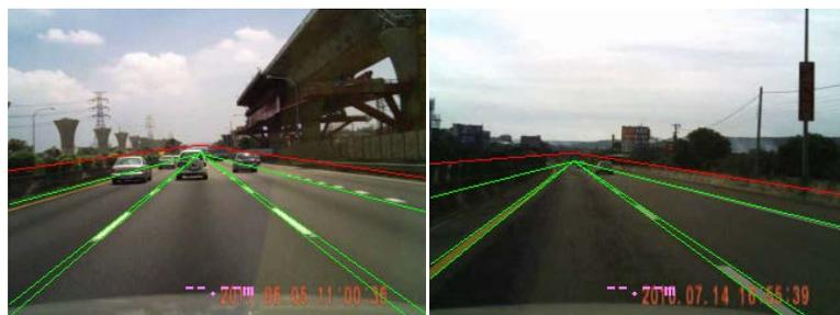
**Figure 1.** Two examples of ROI setting based on the detected lane marks.
