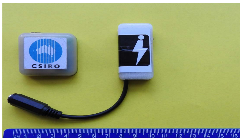
Figure 3. An original (left) and a newer transceiver employed with the automated scoring technology.
