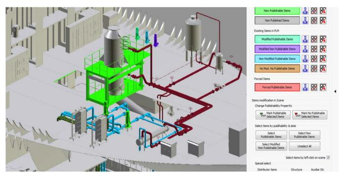
Figure 2. Integration between FORAN and a Project Lifecycle Management tool [2].
