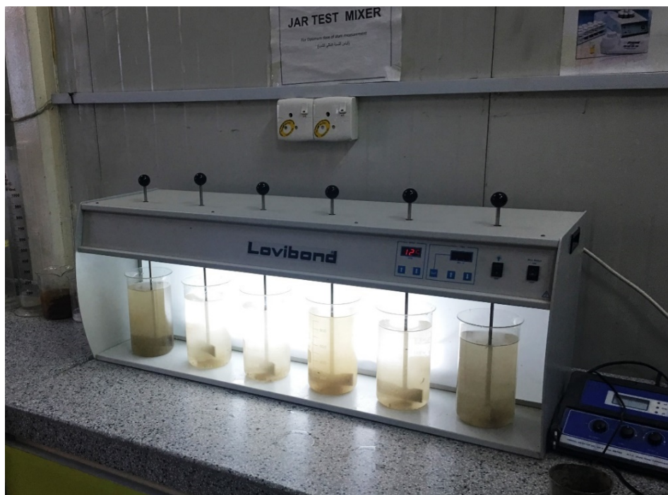
Figure 3. An ordinary jar test apparatus for treatment of turbid water by natural coagulants.
