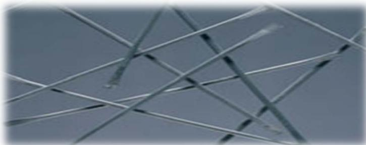
**Figure 1.** Steel fibers.
