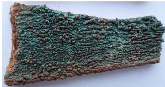
Figure 3. Sample from the copper refinery with copper and corroded products.
