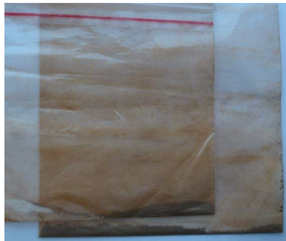
Figure 4. Some corrosion products gathered from the cathode plate and its surrounding.
