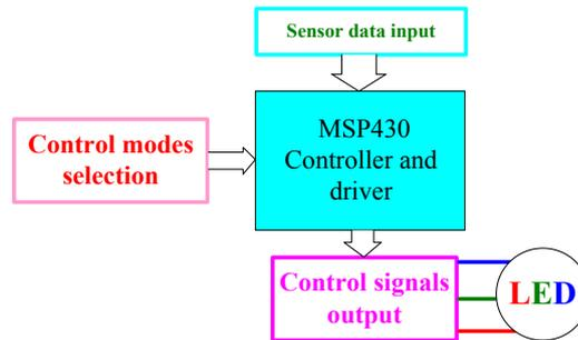
**Figure 1.** Control system block diagram.
