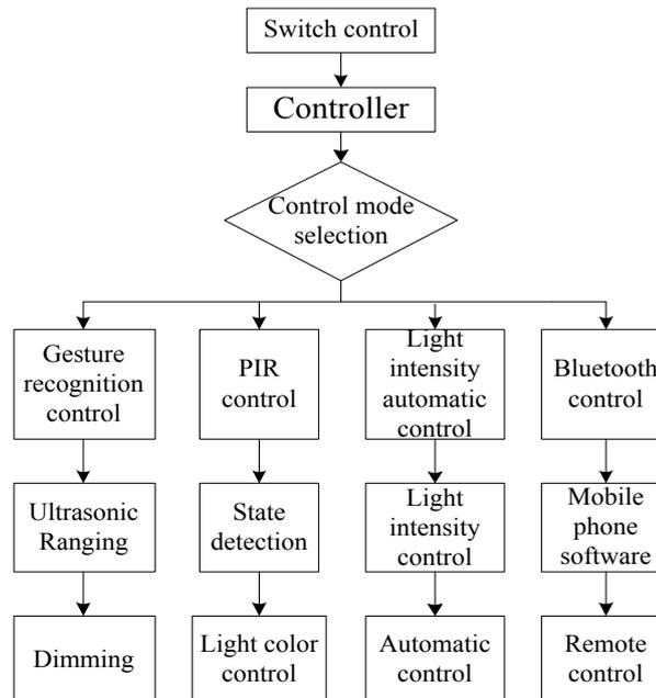
**Figure 2.** The implementation of multi-mode control case diagram.
