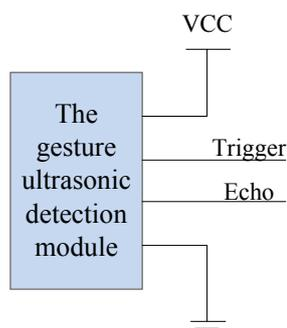
**Figure 3.** The gesture ultrasonic detection module interface circuit.
