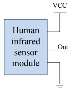
Figure 4. Human infrared sensor module interface circuit.
