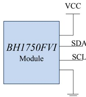
Figure 5. Light intensity detection module interface circuit.
