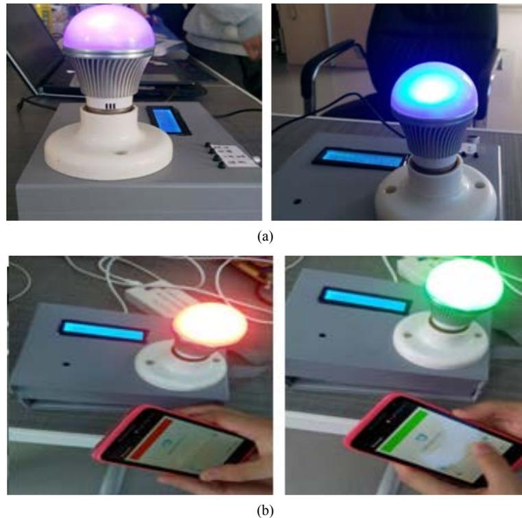
**Figure 10.** Prototype control test results. (a) The human body sensing automatic light change; (b) Bluetooth control lights change.
