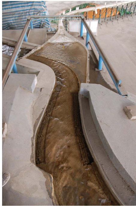
Figure 3. Physical model of the Yuanshanzi Diversion Work (scale: 1/100).
