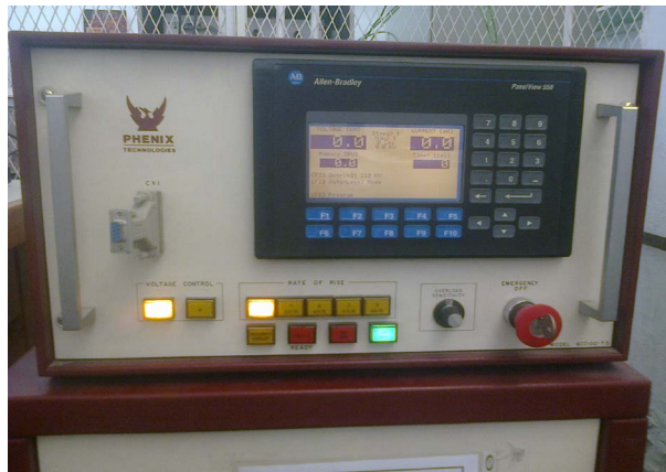
Figure 11. Dielectric test set for dielectric breakdown measurement.
