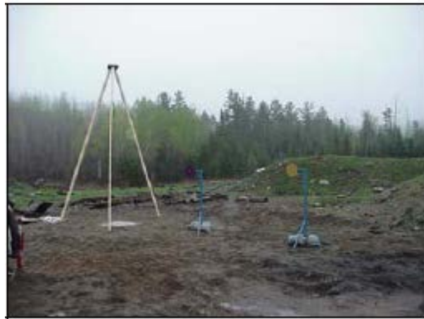
Figure 2. Test specimen with the tripod holding the explosive charge.
