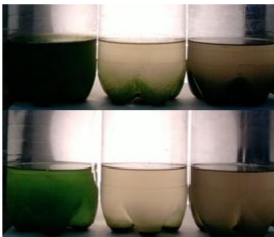
Figure 1. On the picture's upper part is the result of stopping the CO 2 feed, on the under part is the result of flow choke with CO 2 .
