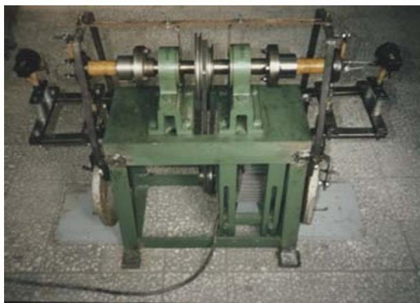
**Figure 4. The bending, fatigue experiment device.**
