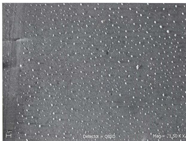
**Figure 2.** SEM image of the ZnO solid spheres obtained using HMTA as SDA and deposited on Si (100) Substrates.
