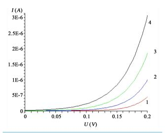
**Figure 1.** CVC p-n-junction at different electron temperature. 1— $T_e = 300 \text{ K}$ , 2— $T_e = 350 \text{ K}$ , 3— $T_e = 400 \text{ K}$ , 4— $T_e = 450 \text{ K}$ .
