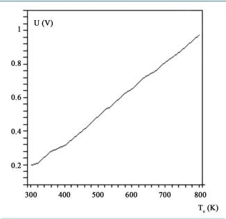
**Figure 3.** The dependence of the open circuit voltage of the electron temperature.
