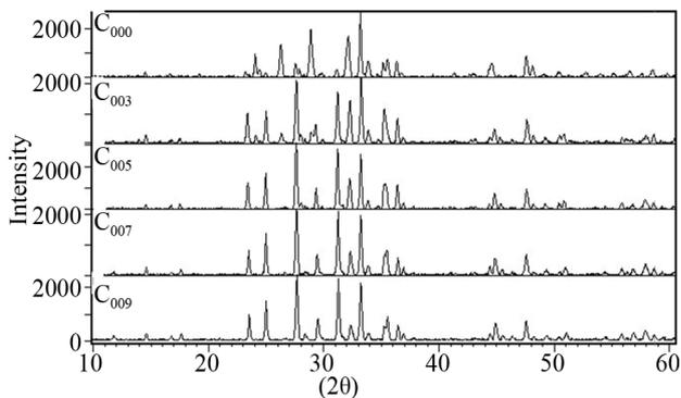
**Figure 4.** XRD patterns of C<sub>000</sub>, C<sub>003</sub>, C<sub>005</sub>, C<sub>007</sub> and C<sub>009</sub> samples after the final stage of the heat treatment.
