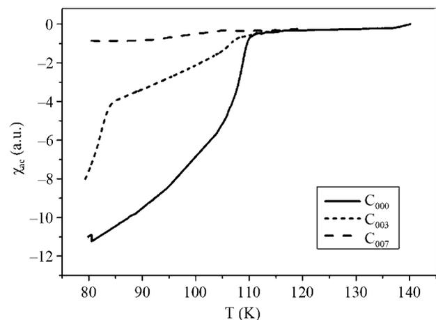
**Figure 6.** The temperature dependence of the real part of AC susceptibility for the C<sub>000</sub>, C<sub>003</sub> and C<sub>007</sub> samples.
