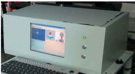
Figure 3. Embedded laser beam quality analyzer.
