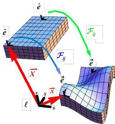
**Figure 1.** In this figure,  $\hat{\ell}$  illustrates the observer coordinate system.  $\mathcal{F}_{ij}$  is the mapping defined at each point in space from the  $\mathbf{X}$  point location before the deformation to the same point  $\mathbf{x}$  after the deformation. Any local coordinate system before the deformation,  $\hat{e}$ , is mapped into a new local coordinate system after the deformation,  $\hat{e}$ .
