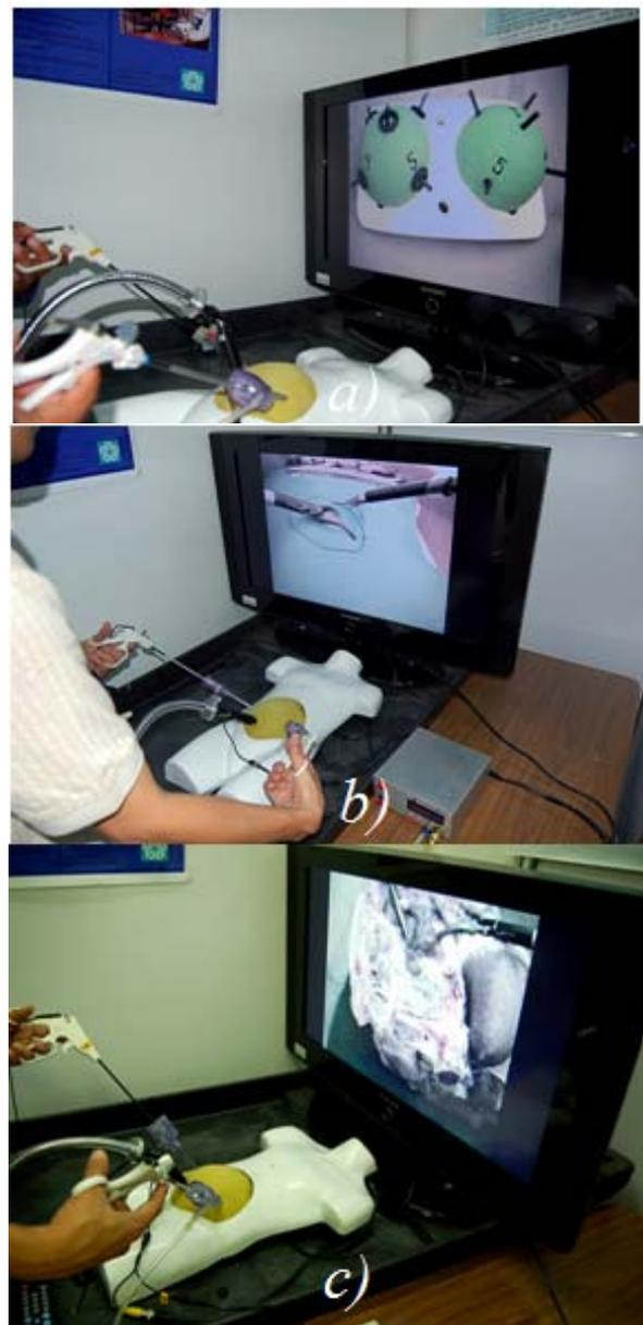
Figure 4. Tasks inside the pressurized chamber: a) Transferring rubber rings; b) MISTELS cutting task modality; c) Animal model dissecting.
