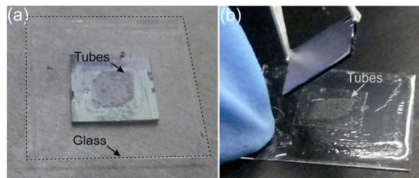
**Figure 2.** (a) GaAs sample placed on the glass substrate (black dashed line); (b) Separation of the glass substrate and the GaAs substrate with tubes lying on the glass substrate. The tubes on the GaAs substrate are released and transferred tubes on the glass substrate.
