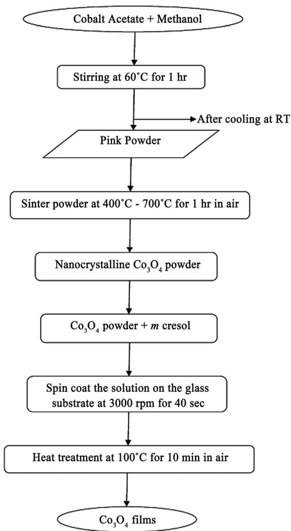
**Figure 1.** Flow diagram for Co<sub>3</sub>O<sub>4</sub> films prepared from the sol-gel process using the spin-coating method.
