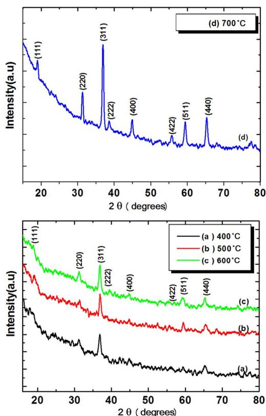
**Figure 2. X ray diffraction patterns of Co<sub>3</sub>O<sub>4</sub> films at different annealing temperatures.**
