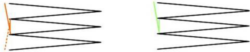
Figure 3. Left: an incident light ray impinging at a large angle indicated by a solid line is reflected twice before being emitted from the absorber (dotted line). Right: a thermal radiation ray emitted with the same spatial and directional parameters as the incident light ray (shown in the left part of the figure), but travelling in the opposite direction.
