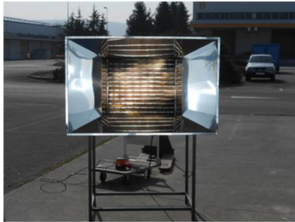
Figure 5. The solar-air heat exchanger illuminated by the concentrated sun light from the Linear Mirror II system.
