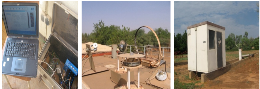
Figure 2. The devices are installed on the roof of the building of the CNES and the shelter of protection of the base of data recording on the spot.
