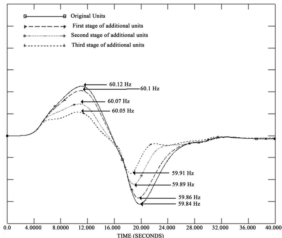
**Figure 3.** The system frequency variation under different additional units (wind power is above 1350 MW).
