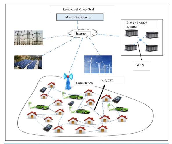
Figure 2. Architecture of SCADA control and communication network with ACT in residential microgrid.
