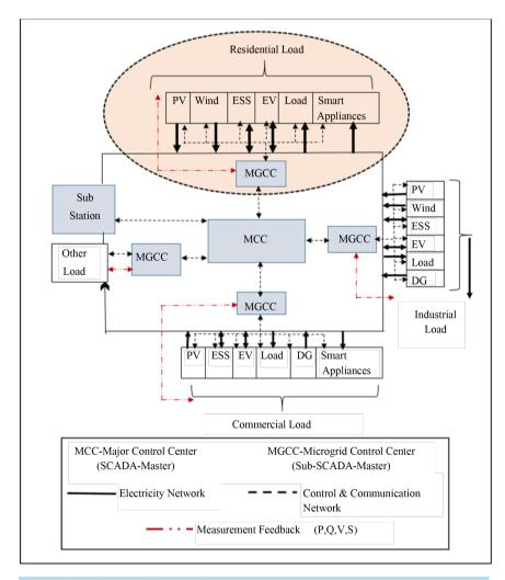
Figure 1. Architecture of MMEMS.
