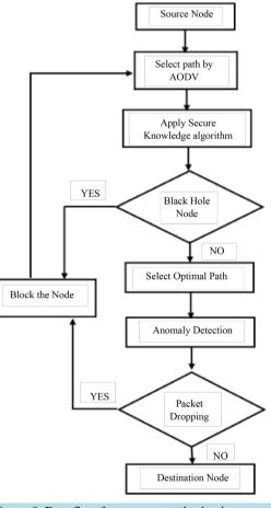
Figure 3. Data flow from source to destination.
