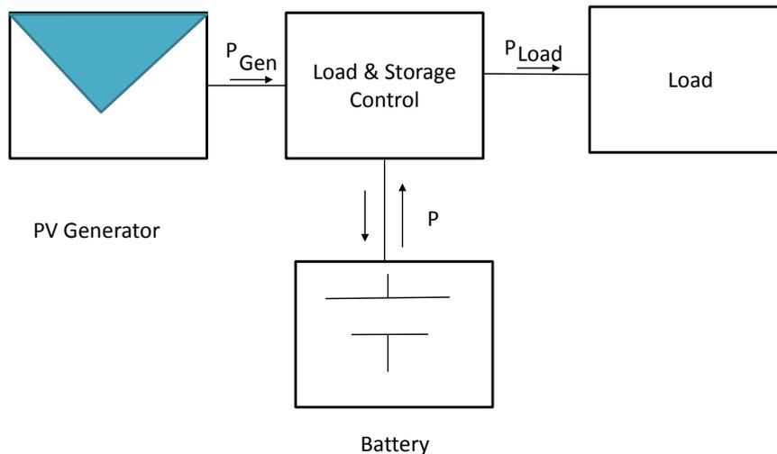
**Figure 2.** Schematic diagram of a PV power system with battery storage.
