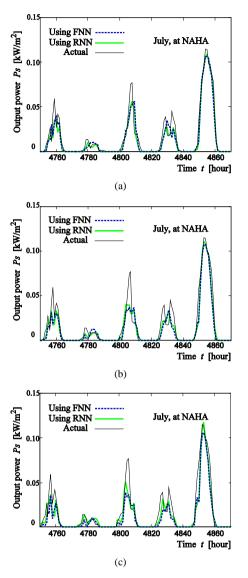
Figure 10. Forecast results of several hour ahead power output for PV system (Jul., 2000). (a) 1 hour ahead; (b) 2 hour ahead; (c) 3 hour ahead.
