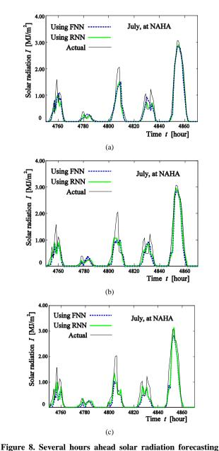
Figure 7. Several hours ahead solar radiation forecasting (Jun., 2000). (a) 1 hour ahead; (b) 2 hour ahead; (c) 3 hour ahead.
