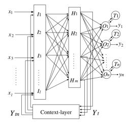
Figure 4. Recurrent neural network (Elman type).
