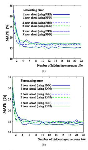
Figure 6. Forecast error to number of hidden-neurons. (a) Using past data of temperature; (b) Using forecasted data of temperature.
