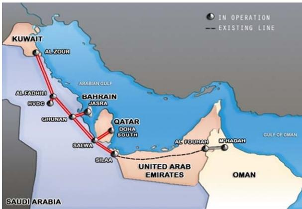
Figure 4. GCC power grid interconnection project [10].
