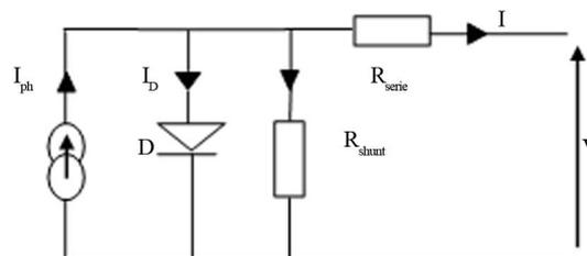
Figure 2. Equivalent circuit of a PV cell.
