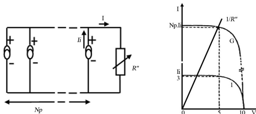
Figure 7. Group of cells in parallel [11].
