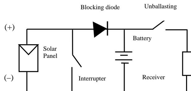
**Figure 11. Diagram of a shunt regulator [12].**
