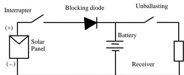
**Figure 10. Diagram of a control series.**
