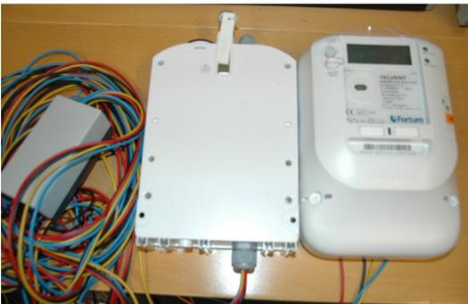
Figure 6. Smart meter and concentrator setup.
