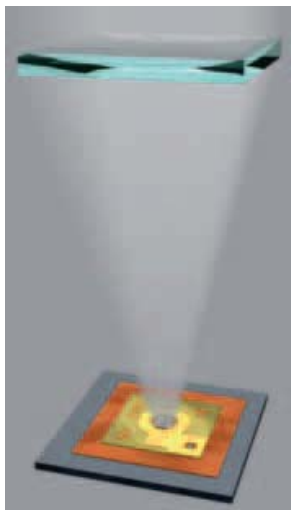
Figure 6. Schematic illustrating the operation of a multi-junction solar cell in a concentrator system.
