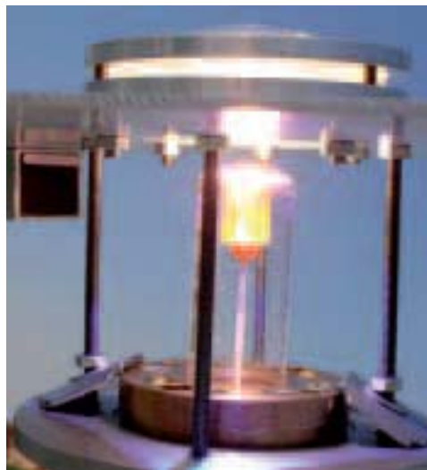
Figure 7. Emitter heated up by the sun through a concentrator system.
