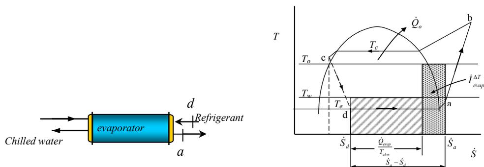
$$\dot{I}_{evap}^{\Delta T} = \dot{m}_r T_o \left[ (s_a - s_d) - \frac{(h_a - h_d)}{T_{sw}} \right] \quad (34)$$
