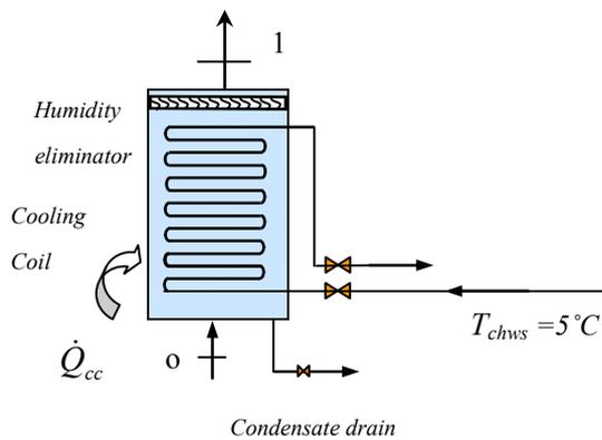
$$i_{cooling\ coil} = \dot{m}_a (1 + \omega_1) T_o (s_o - s_1) + \dot{Q}_{out} \tag{32}$$
