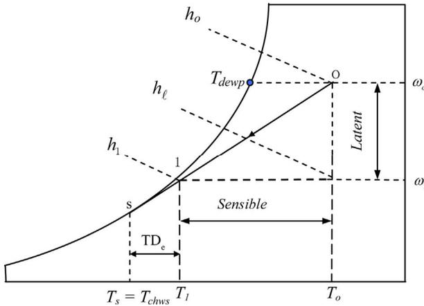
Figure 3. Moist air cooling process before GT compressor intake.
