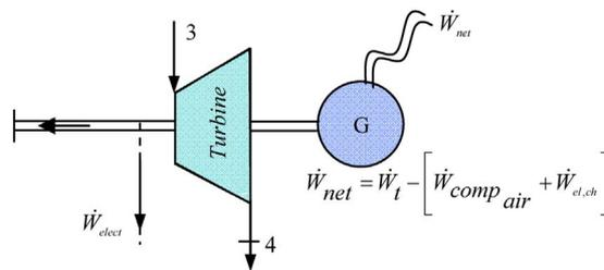
$$\dot{i}_{gas\ turbine} = \dot{m}_a (1 + f + \omega_1) T_o \left[ c_{pg} \ln \left( \frac{T_4}{T_3} \right) - R_g \ln \left( \frac{P_4}{P_3} \right) \right] \quad (26)$$
