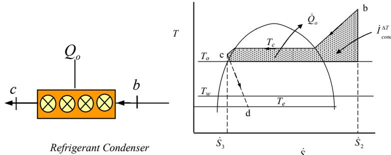
$$i_{cond}^{\Delta T} = \dot{m}_r T_o \left[ (s_c - s_b) + \frac{(h_b - h_c)}{T_o} \right] \tag{29}$$
