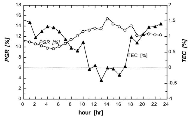
Figure 7. Variation of gas turbine PGR and TEC during 18<sup>th</sup> August operation.
