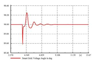
Figure 12. Smart Grid voltage angle during integration of DGs in degree.
