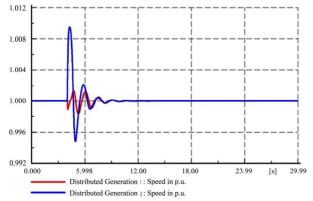
Figure 9. Distributed Generation speed in p.u during integration to Smart Grid.
