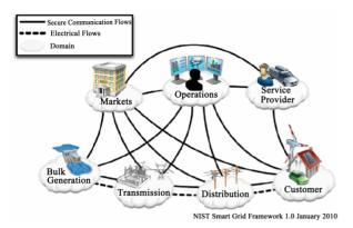
Figure 1. Smart Grid topology network [9].
