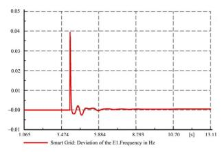
Figure 11. Smart Grid frequency total deviation during integration of DGs in Hz.
