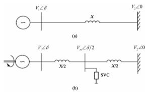
Figure 3. Simplified power systems (a) without SVC and (b) with SVC [14].
