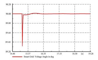
Figure 15. Smart Grid voltage angle during 3 phase fault in p.u.
