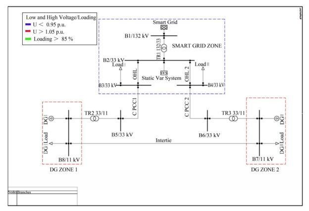
Figure 5. Smart Grid topology network.
