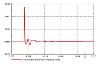
Figure 10. Smart Grid frequency during integration of DGs in Hz.
