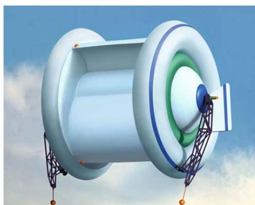
Figure 9. Some proposals of aerial wind turbines. The magnenn power wind turbine, called MARS, differs from a kite-style wind power system in that it's held aloft by helium rather than relying on the force of wind. Lack: One cannot use a strong wind and high altitudes.
