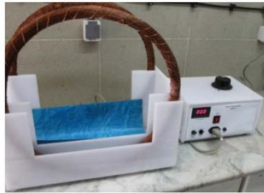
**Figure 1.** A view of the electromagnetic devices (small animal cage place: on the blue section).
