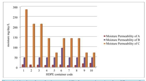
Figure 1. A bar chart of rate of moisture permeability for ten tested containers from different suppliers *i.e* coded supplier A, B and C.
