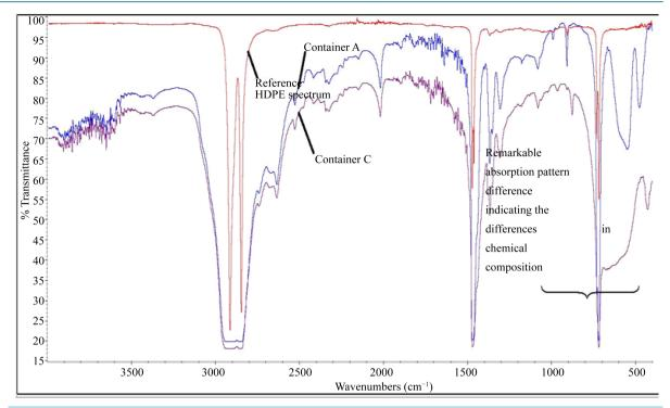
Figure 2. Spectra of plastic container from supplier A and C over-laid together with the reference HDPE spectrum, all scanned from  $4000 - 400 \text{ cm}^{-1}$  with KBr as a detector and a total of 16 scans were collected.
