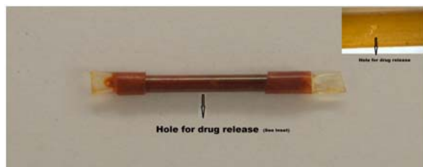
Figure 1. The drug delivery system with microhole on the surface. Hole diameter = 200 \mu m; Tube diameter = 1.8 mm; Tube length = 20 mm. The size of the device and the perforations can be scaled to fit the need of the therapeutic application [12].
