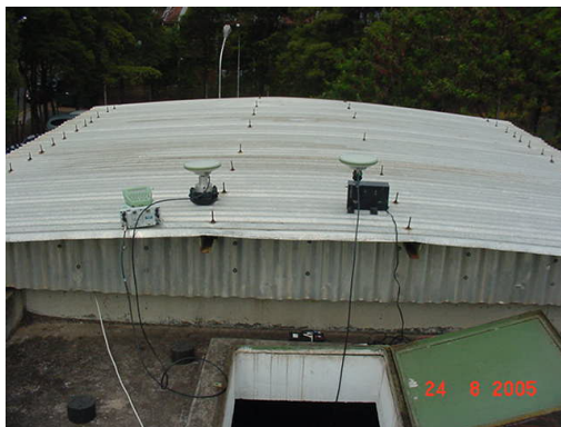
Figure 1. The antennas at the EESC - USP Campus and the rover antenna is mounted over the EMO.
