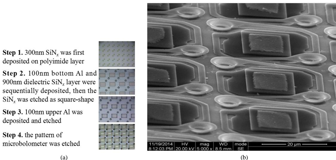
**Figure 1.** (a) The left indication shows the process steps for fabrication of MM-based microbolometers, the right pictures are the optical images for the sample after each steps, (b) the top view of SEM image of the as-fabricated array.
