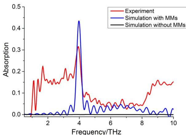
**Figure 3.** Experimental (FTIR) and simulated results of the microbolometers with and without MMs.
