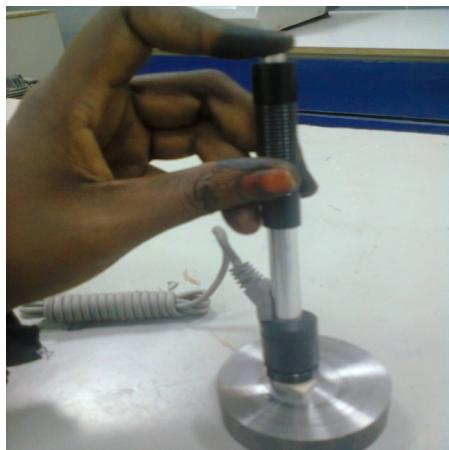
**Figure 3.** The method of hardness measured.
