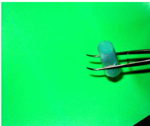
Figure 3. A photo of conductive, transparent and flexible PET.
