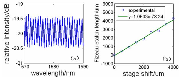
**Figure 3.** (a) Interference signal spectrum (part 1 in Figure 1), (b) Relationship between the stage shift and the length of Fizeau cavity.
