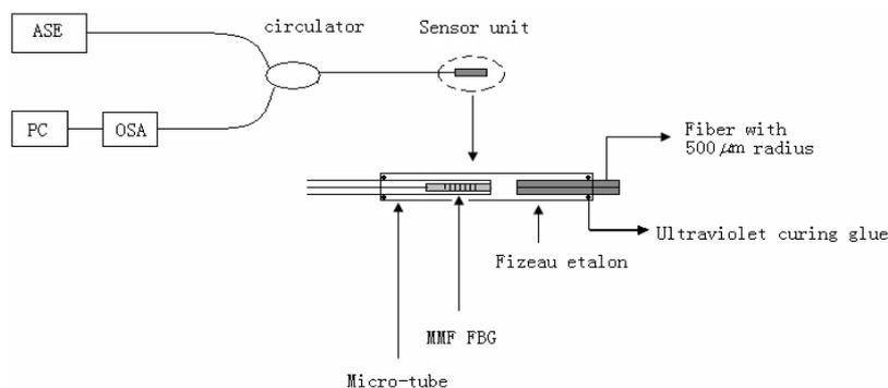
**Figure 1.** A GI MMF based sensor unit and its demodulation scheme.
