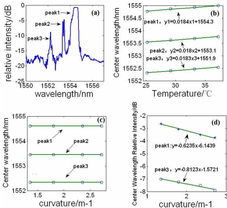
**Figure 4.** (a) The signal of MMF-FBG (part 2 in Figure 2), (b) The temperature response of the MMF-FBG, (c) center wavelength with the change of curvature, (d) the curvature response of the GI MMF-FBG.
