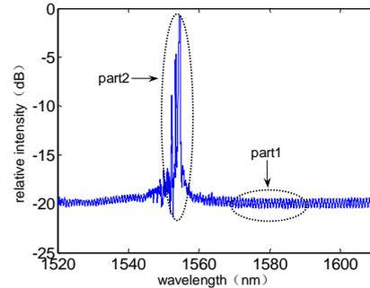
**Figure 2.** A signal of the GI MMF based sensor unit.
